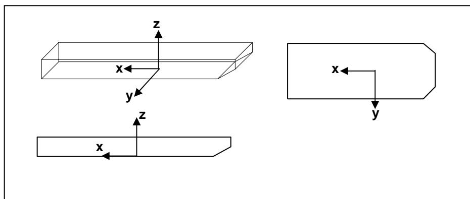
Figure 3.1 Definition of marine co-ordinate system
